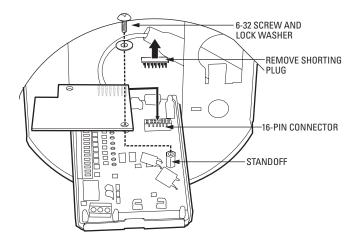
Figure 8. Spectra III/Spectra IV Back Box Circuit Board
